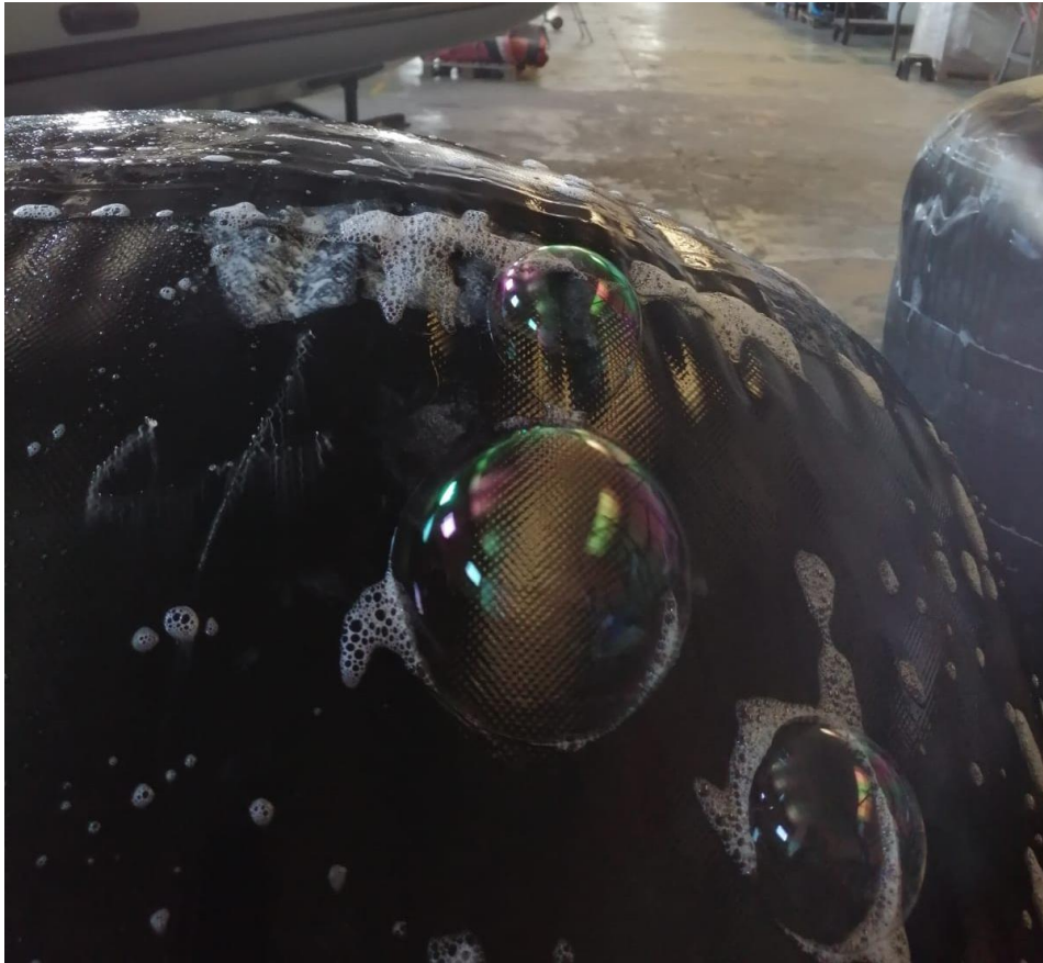
Fender 4 (Diameter 90 x 95cm) – Bad conditions, air leaking through glued seams
