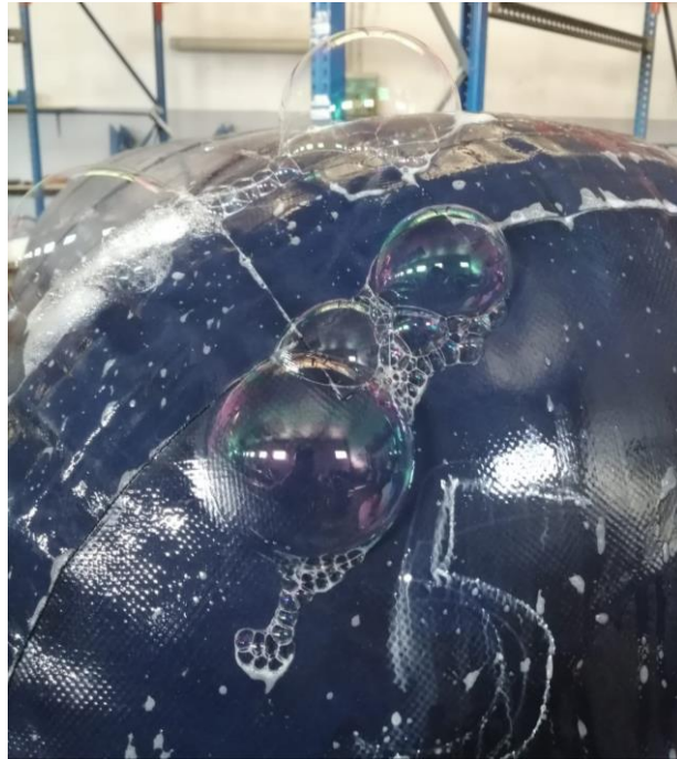
Fender 5 (Diameter 62 x 122cm) – Bad conditions, air leaking through glued seams
